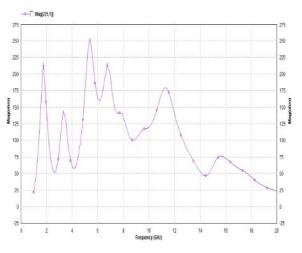
Graph between Frequency and Magnitude Input Impedance of Sierpinski Carpet Antenna Frequency vs. Various Efficiency Plot of Sierpinski carpet antenna
