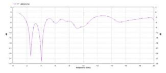
Fig. Return Loss Graph of 1<sup>st</sup> Iteration Sierpinski Carpet Antenna
