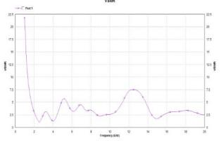
**Fig VSWR Plot of Sierpinski Carpet Antenna Input Impedance Plot of Sierpinski carpet antenna** I expect pure impedance at frequencies where the patch resonates, and see table 5.3 and figure 5.3
